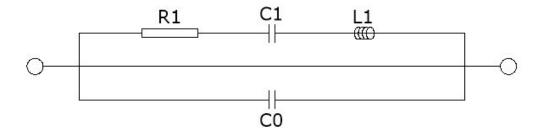
This circuit consists of L1 (motional inductance), C1 (motional capacitance), and C0 (shunt capacitance). While all parameters can be adjusted through design, they are interconnected, meaning a change to one will affect the others.
